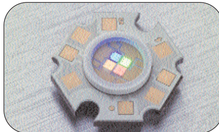
Figure 2. Shows the ACULED High Performance RGB LED (with 4 chips) in COB technology
