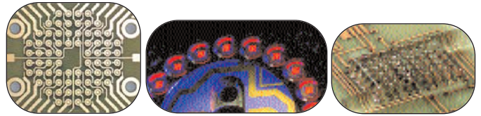
Figure 5. Shows several COB solutions with different types of optical beam shaping elements
