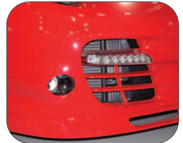
Figure 2. LEDs are being implemented into vehicles for turn signal and side marker illumination
