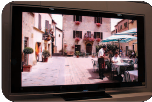
Figure 3. Premium HDTVs such as the SONY 70XBR will continue to be backlit by RGB LEDs with color gamut > 105 percent NTSC
