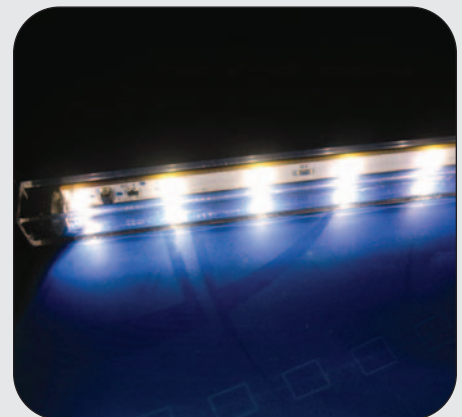
DDP replaced the 24 VAC Tivoli lights under the armrest with six warm white, surface-mount LEDs and a custom PC board and acrylic housing.
