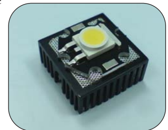
Figure 3. Temperature measurement point on Moonstone LED package.
