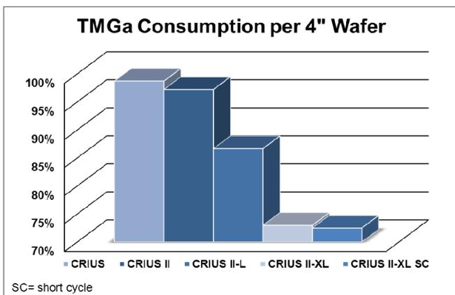
Fig. 2: Trimethylgallium (TMGa) consumption per 4" wafer for Close Coupled Showerhead® reactors
