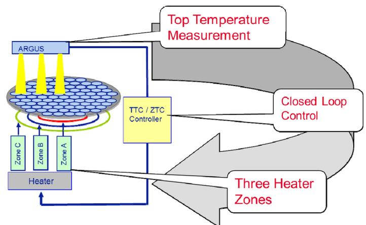
Fig. 3: Schematic of the TTC (Top side Temperature Control) in a CRIUS® II-XL MOCVD reactor
