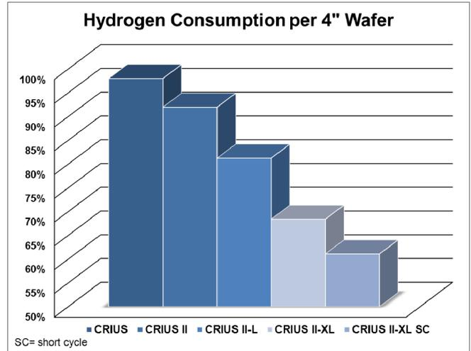
Fig. 5: Hydrogen consumption per 4" wafer for Close Coupled Showerhead® reactors
