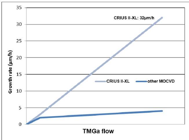
Fig. 4: Growth rate of CRIUS® II-XL and other MOCVD reactors as a function of the TMGa flow
